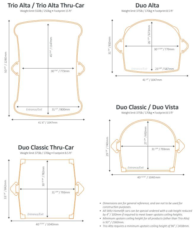
• Local code requirements may limit the weight for the Trio Alta / Trio Alta Thru to 500 pounds (227kg).
