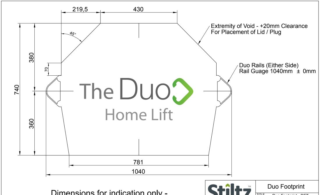
Dimensions for indication only -Use template for accurate marking of void
